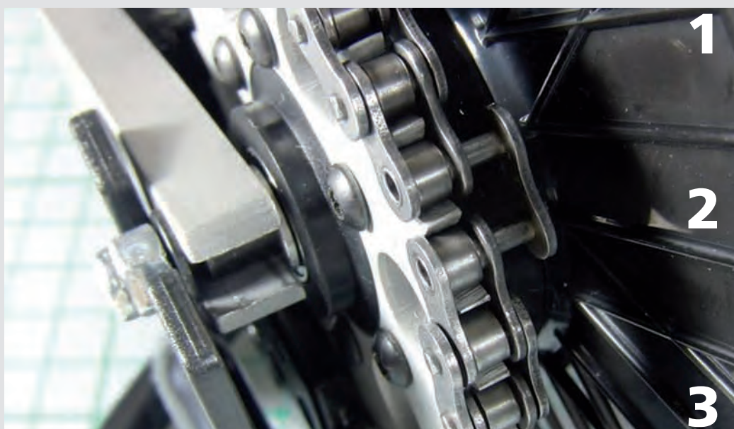
Korrekt monteret/ Correct installation.
